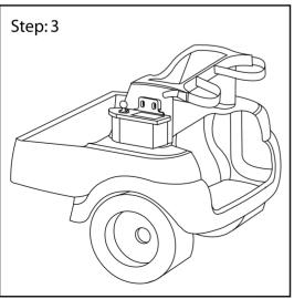
Step: 3 Now with Club and Ball Washer unit right side up, put the Bevel Edge of Part "CC2004" in groove edge of fender on Golf Cart. Now use the two black M6 button head Allen Screws with 2 - 3/16" black flat washer to secure bracket to rear of Golf Cart. Using the two Mounting Holes on side panel of Golf Cart.
