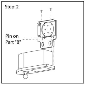
Step: 2 Turn Club & Ball Washer unit upside down. Now insert the four pins on Part "B" into the four holes on the underside of Lid. Now using the two black 3/4" #10 Phillips Truss head screws, locate two holes on the bottom of the Ball Washer Case and secure Part "B" of bracket to bottom of Ball Washer.
