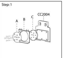
Step: 1 Insert 4 1/4-20 hex bolt through outside set of holes on Part "A". Snap Part "A" into Part "B". Insert bolts through outside set of holes on Part "C". Now on Part "CC2004" from back side start four 7/16" nuts into hexed shaped holes, now tighten bolts.
