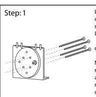
Locate a post or support bracket on the rear of your golf cart to mount your Golf Ball Washer. Use either the four inside holes on part A, or the outside holes on part A to insert bolts into.
