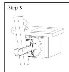
Slide the "optional" part D onto the four bolts using either the four inside holes, or the four outside holes.
