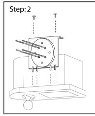
Turn your Club & Ball Washer unit upside down and locate four holes on the under side of the lid. Insert the four fingers on part B into these holes. Take two #10 3/4" black screws, and secure them into the screw bosses on the bottom of Club & Ball Washer Unit.
